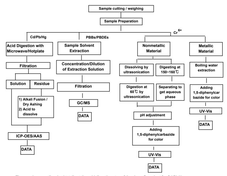
The samples were dissolved totally at the acid digestion step of the above flow chart for Cd,Pb,Hg Section Chief : Taehee Kang
